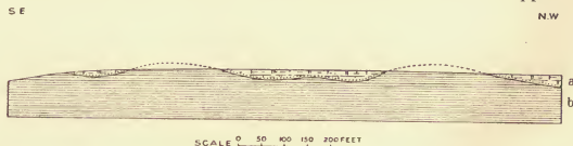
FIG. 6. Diagrammatic section north-east of Haslingfield, Cambridgeshire. (From W. H. Penning and A. J. Jukes-Browne, 'The Geology of the Neighbourhood of Cambridge', Mem. Geol. Surv. , 1881, p. 37, Fig. 7.) a. Chalk Marl. b. Gault.
